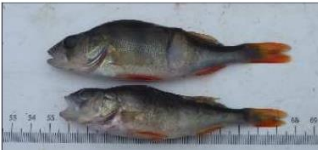
Figure 3.7 Two dead perches with severe abrasions in the rump area, directly after conducting the test.
