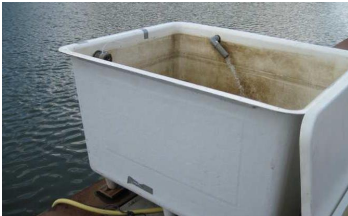
Figure 2.4 One of the tanks flushed with fresh water from the Merwede Canal.
