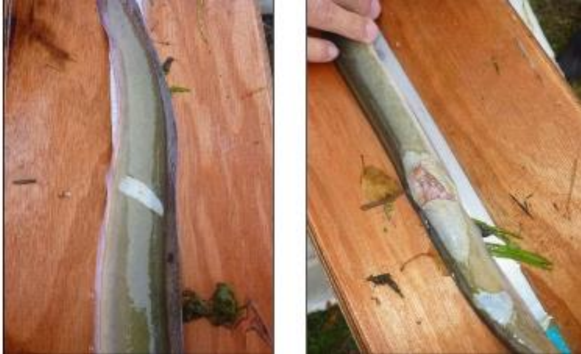
Figure 3.6 Samples of slight damage (left) and irreparable damage (right) directly after conducting the test.
